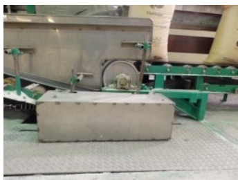
Conveyor drums protect- ed with safety guards
